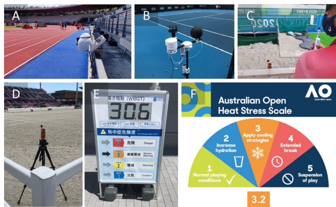
Figure 1 Environmental condition monitoring and reporting. Panels A and B: devices specifically developed for World Athletics and for the Australian Open Tennis tournament, respectively. These are the recommended solutions. Panels C and D: commercially available units used on the field of play. It is not recommended to use a hand-held device (panel C) when the device was stored in the shade between measurements as it led to a 2°C error compared with the stationary device. The device should be fixed on a tripod prior to the event to allow for some time to equilibrate to the environment for accurate measures (panel D). Panel E: the display of wet bulb globe temperature (WBGT) monitor and risk category prepared by the Tokyo Organising Committee of the Olympic and Paralympic Games. This display may confuse the athletes as most do not know the WBGT and may misinterpret it as air temperature. Furthermore, the colour coding was different from what has been implemented by various international federations. Panel F: colour-coded 1–5 Heat stress scale developed for the Australian Open Tennis tournament by the University of Sydney. It provides the actual index (value) and the corresponding recommendation. This feedback method provides a clear message for athletes and is recommended.
